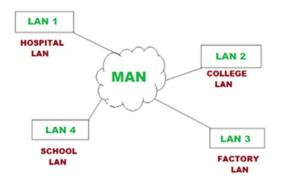
The fault tolerance of a MAN is less and also there is more congestion in the network. It is costly and may or may not be owned by a single organization. The data transfer rate and
